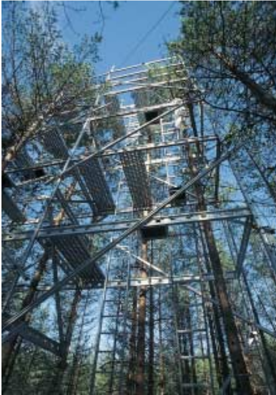
Figure 8–1 The observation tower at Hyytiälä Forestry Field Station of the University of Helsinki. The installation, SMEAR (Station for Measuring Forest Ecosystem-Atmosphere Relations) gives continuous information on interactions between trees and atmosphere, air quality and aerosols.
