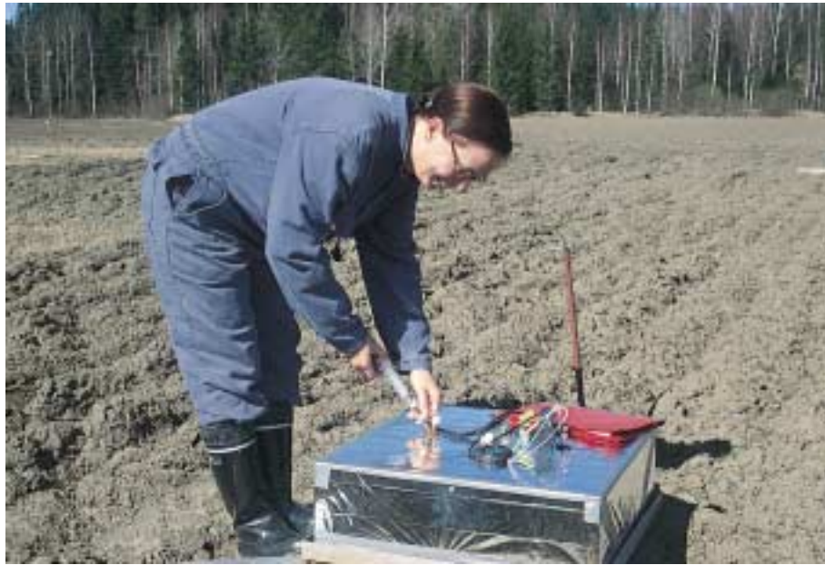
Figure 6–3 A FIGARE measuring site of the Agrifood Research Finland (MTT) at Jokioinen, south-western Finland. Methane and nitrous oxide emissions were measured in all seasons in 2000–2002.
